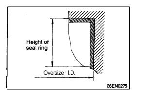
(2) Rebore the valve seat hole in the cylinder **head** to' **a** selected oversize valve seat diameter.
