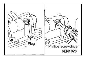
(4) **Insert** a Phillips screwdriver [shank diameter 8 mm **(.31** in.)] through the hole.
