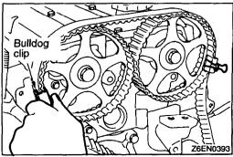
(5) Thread the timing belt over the intake side camshaft sprocket and fix it at indicated position by a bulldog clip.
