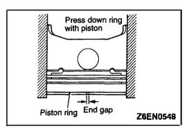
(3) Install the piston ring into the cylinder bore. Force it down with a piston, its crown being in contact with the ring, to correctly position it at right angles to the cylinder wall. Then, measure the end gap with a feeler gauge. If the ring gap is excessive, replace the piston ring.
